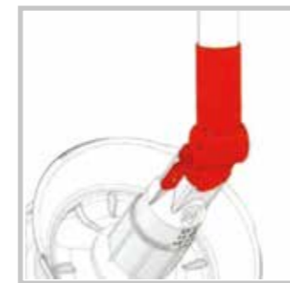
Articulation between feeder and lowering (combination 10+14)
